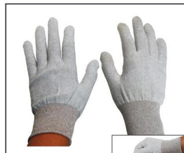
A properly grounded operator can touch a charged ESD sensitive device and a damaging ESD event can occur (Charged Device Model). Increasing the electrical path's contact resistance is one way to control the speed of the discharge and reduce the possibilities of damage. A good way to accomplish this is by wearing static dissipative gloves.
